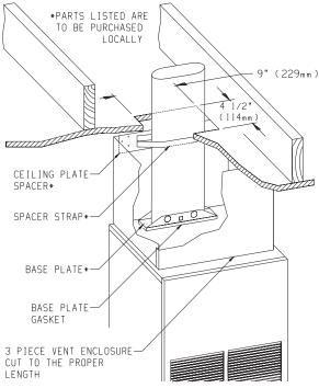
ALL CONNECTIONS MUST BE MECHANICALLY MADE AND LISTED CLEARANCES MAINTAINED
